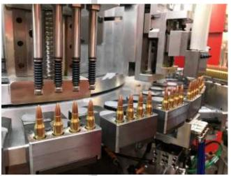
100% Electronic control of the bullet height (AOL) and the primer height, both are measured not just as ok or not ok, their measure is stored in the machine database, pieces by pieces, allowing the statistical analysis.
